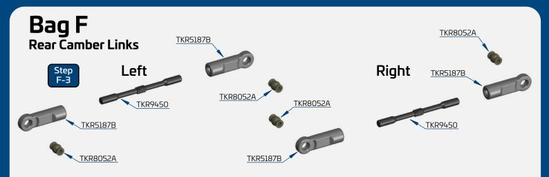
Build Tip: Use some grease or Chapstick on the threads to help prevent "pop-off" when adjustments are being made.
