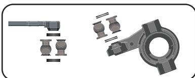
Bump steer is a front suspension tuning option commonly used to change steering characteristics over rough and loose terrain. Bump steer occurs when a vehicles front toe angle changes as the suspension compresses or rebounds, which affects how parallel the front wheels are.
