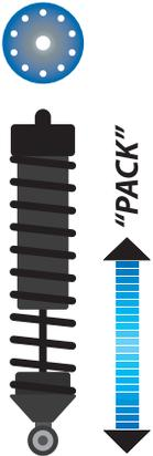
Shock pistons come in a variety of hole size/number of holes variations. The size of the holes or number of holes affect shock damping by altering the flow of oil through the holes. More holes or larger holes give softer damping. Fewer holes or smaller holes give harder damping.
