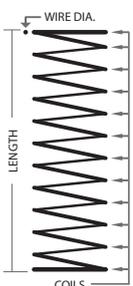
Spring tension determines how much the shock resists compression, which is commonly referred to as the "hardness" of the spring. Different spring tensions determine how much of the vehicles weight is transferred to the wheel relative to the other shocks. Spring tension also influences the speed at which a shock rebounds after compression. Spring tension is usually rated in a "spring weight"; higher spring weights are stiffer, while lower spring weights are softer.
