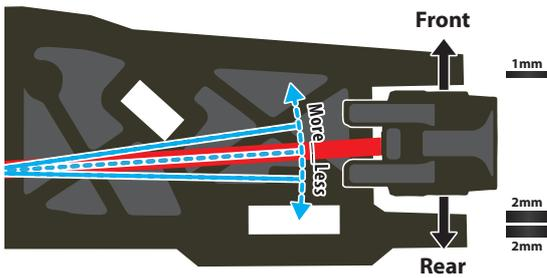
Changes to wheelbase can have a dramatic effect on the handling of your vehicle, since it adjusts the distribution of weight on the rear wheels, which adjusts traction. By shortening the wheelbase at the rear of the vehicle, you're placing more weight over the rear wheels, which results in more rear traction. By lengthening the wheelbase, the vehicle feels more stable and the longer vehicle handles bumpy sections easier.
