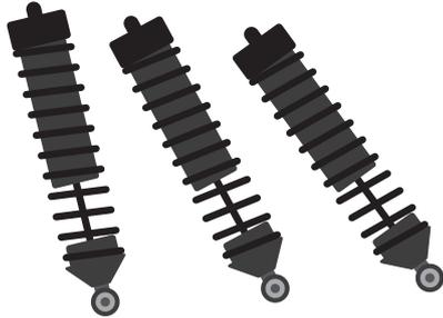
You can manipulate the handling characteristics of the vehicle by changing the shock mounting position. Leaning the shocks at different angles and moving the shock closer or further from the centerline of the vehicle will have different effects on handling.
