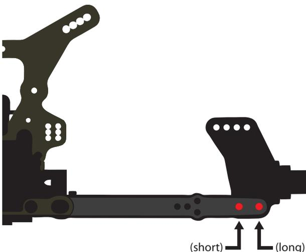
Rear arm length can be adjusted on our kits to suit various driving styles or track conditions by simply moving the rear outer hinge pin. This will change the point in which the rear hub will articulate.
