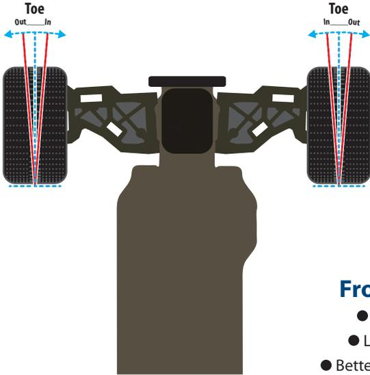
Toe in and toe out are terms used to describe the angle in which the wheels point when looking down at them from the top of the vehicle. Toe is used to stabilize the vehicle at the expense of traction. Front wheels can be toed in or out to suit various situations. Rear wheels should only have varying degrees of toe in.
