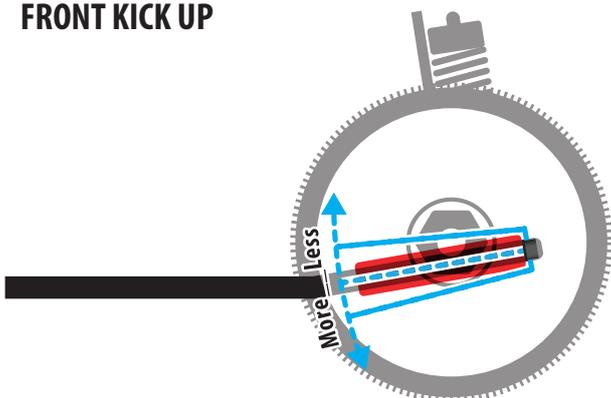
Front kick-up is used to adjust the amount of weight transfer to the front when the vehicle is off-throttle or under braking. Changing the front kick up angle also changes the caster angle (see Caster section).
