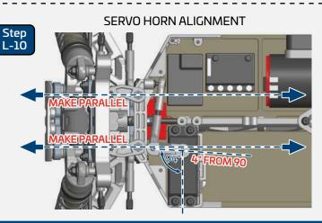
Note: Servo horn should be positioned after trim and sub-trim have been zero'd out. It should be positioned about 4 degrees off parallel from the steering bellcranks.
