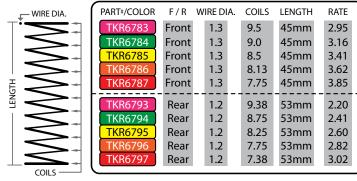
Softer springs will increase traction through the turns by allowing more roll, slow down the responsiveness of the vehicle, and can be better in the bumps. Stiffer springs will increase corner speed if traction is available and will also tend to jump and land better. Once you find a set of springs you like you will typically only change them for tracks with dramatically different conditions.
