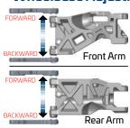
Changes to wheelbase can affect the overall handling of your vehicle, since it adjusts the distribution of weight on the wheels as well as the angle of the driveshafts. Shortening the wheelbase at the rear will give you more steering into a turn and off power, less steering out of a turn and on power. Lengthening the wheelbase at the rear will yield the opposite results.
